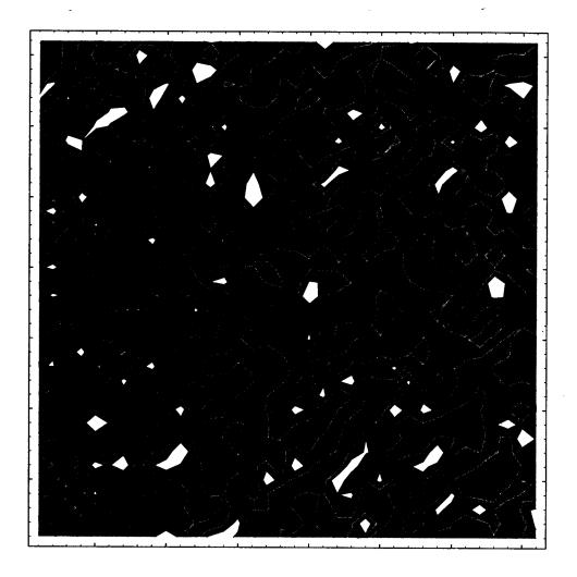
Figure 3.12: The granular temperature field for System IV at a time corresponding to 100 collisions per particle following the initial condition. The shade code is: lighter gray for higher temperatures and darker for lower temperatures. A comparison with Fig. 3.11 shows that regions of higher temperature correspond to regions of lower density and vice versa.
